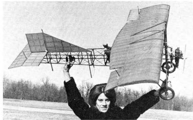
Wing structure is straight-forward. Undercamber causes no big problems. Below: Sun streaming through. You can appreciate your efforts in flight. It brings aviation's history closer to your mind. A magnificent machine.
