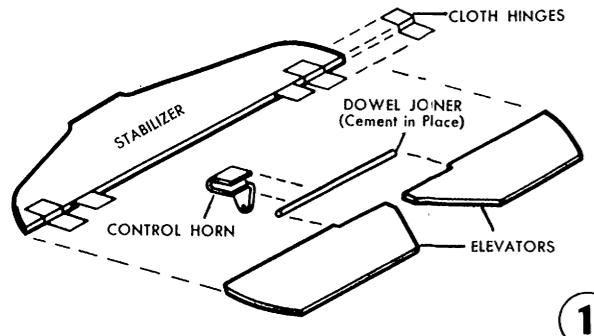
Sand all wood parts with 3/0 sandpaper. Cement the dowel joiner to the elevators and control horn to the left elevator. Hinges  $\frac{3}{8}'' \times \frac{3}{4}''$  are cut from handkerchief cloth and cemented in place as shown.
