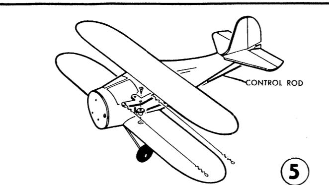
Bend the ends of the bellcrank upward slightly and assemble it, using a  $\#2 \times \frac{3}{8}$  wood screw and the hardwood mount which is then securely cemented in hole in lower wing. Bent end of control rod is inserted in horn and opposite end is bent upward, being sure that proper length is maintained to insure neutral position of elevator and bellcrank.
