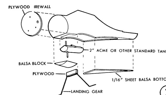
We used an Acme half "A" gas tank with plastic tubing extensions. Cement tank in fuselage using sufficient quantity of cement and being sure extensions are long enough. Then install landing gear  $\frac{1}{2}$ . A soft balsa block is fitted in place under front of fuselage after shaping to fuselage contour. Rear portion of fuselage is covered with  $\frac{1}{16}$  sheet balsa.
