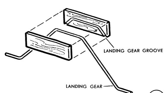
Landing gear is sandwiched between the two plywood parts, fitting it into the grooves in the plywood and cementing well. Finally wrap with thread and apply another coat of cement. Wheels are held on with a fibre washer cemented to end of landing gear.
