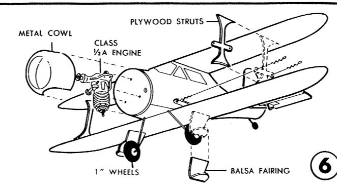
Engine is fastened to plywood firewall with wood screws (either inverted or upright). Install metal cowl using straight pins driven through and into the plywood firewall. Fit and cement wing  $\frac{1}{2}$  in place. Landing gear fairing is cemented under bottom wing allowing sufficient clearance for wheels. Paint entire model white and apply the black decals followed by a coat of glossy quality fuel proofer.
