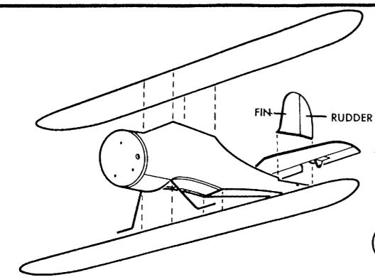
Shape rear of fuselage as shown in side view and fig. A. Cement upper wing to fuselage (wing without hole) and allow to dry thoroughly for several hours. Then cement lower wing (wing with hole) in place, being careful to keep it square with upper wing so that it shows neither positive or negative incidence. Cement fin and offset rudder as shown in fig. A.
