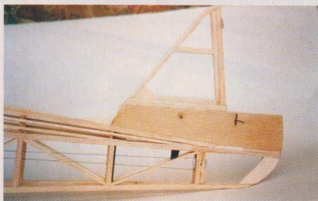
▲ Construction photo 10 - the completed tailplane mount.
