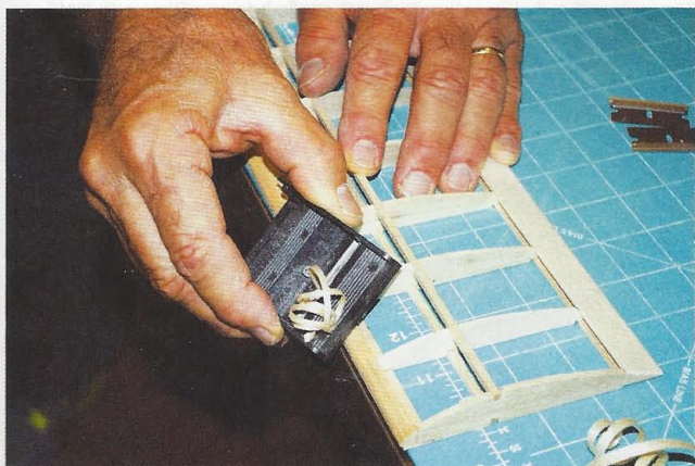
Plane off edges to shape and sand smooth
