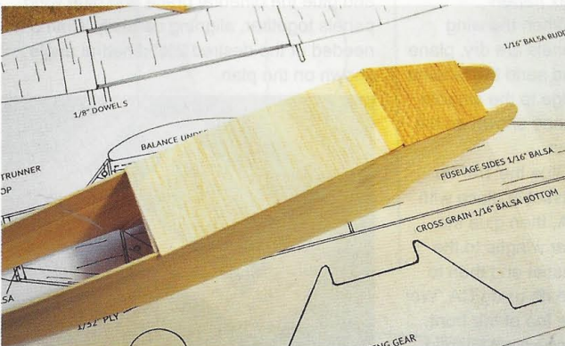
Cross grain 1/16" balsa sheet added to the fus bottom
