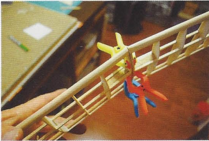
Clamp the wings and allow glue to dry
