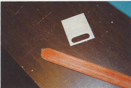
Firewall from 1/32" plywood
