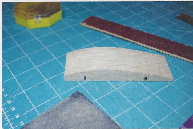
Using the sandwich method sand flush to shape
