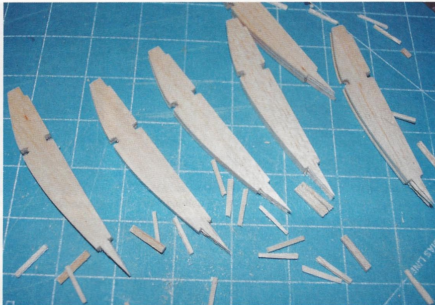
Remove the waste and you should have ribs ready
