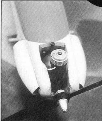
Cox .049 Texaco glow powers the prototype. Cowl cheeks house ballast.
