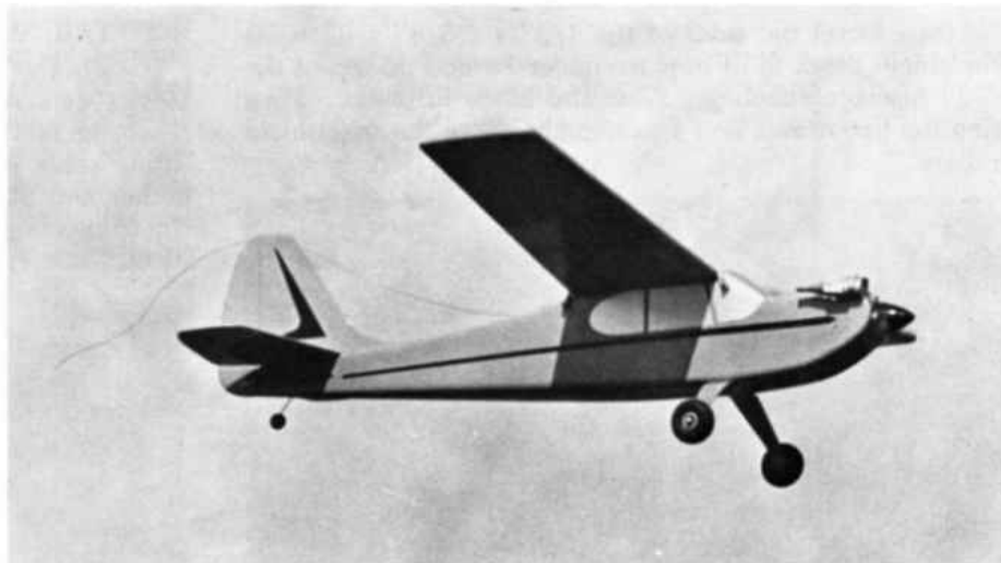
Prototype Scamp #2 on a fly-by. The entire model, including the foam wing, is covered with orange ECONO-KOTE, made by Top Flite. A FUJI .09 engine provides the power.
