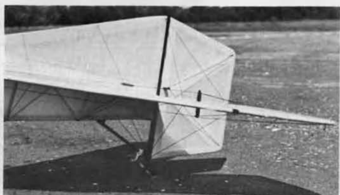
Here again, we can compare the real airplane with the model. What appears to be wide tail structure is really the reinforcing pinked tape over very thin structural members.
