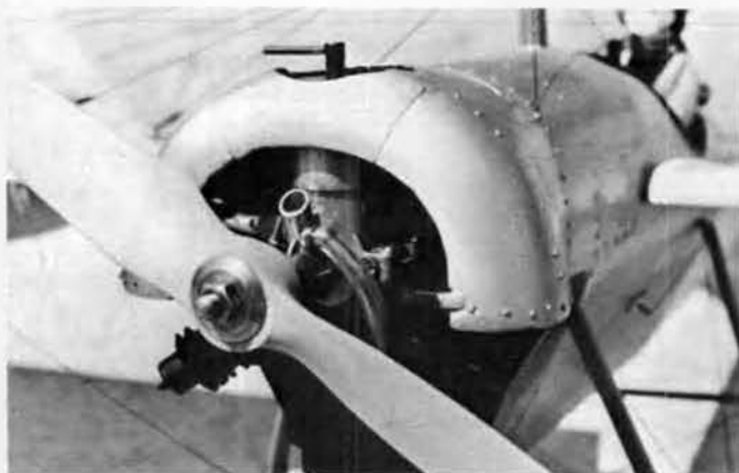
Close-up of engine installation on model, also cowl riveting. Original model used .06 diesel.
