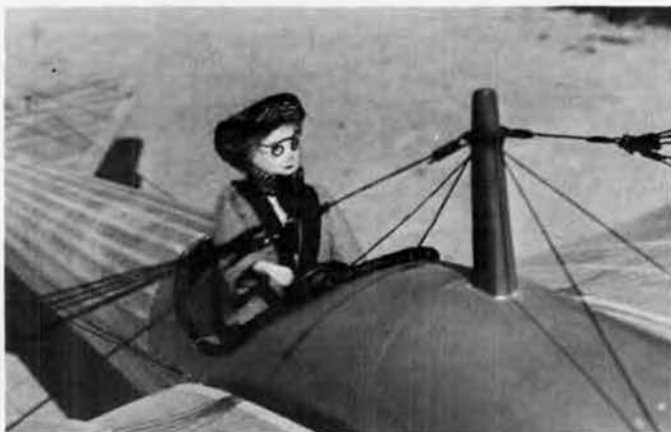
Wing flying and landing wires on model are functional. Original aircraft used wing warping instead of ailerons.
